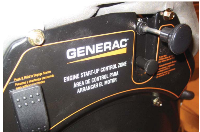
Figure 19 - Full Choke Position
